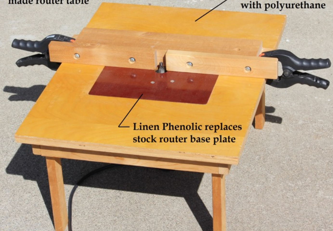
Burt Rosensweig home made router table
